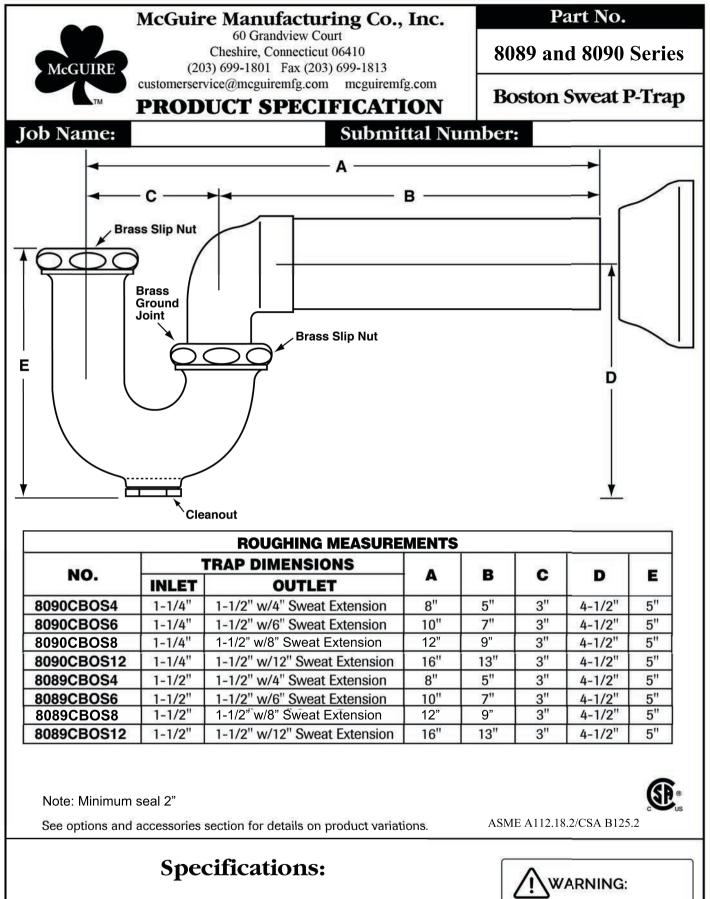
P-Trap shall be chrome plated cast brass body with cleanout, 17 gauge seamless tubular sweat extension, cast brass ground joint elbow, and cast brass slip nuts. No reducing washers. With (shallow, deep, bell) (steel, brass) or (forged brass with set screw) flange.
