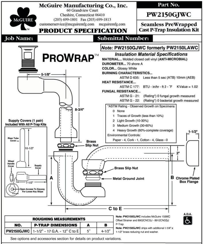
Seamless PreWrapped Adjustable Cast Brass P-Trap Kit with PreWrapped offset grid drain. Furnished with McGuire cast brass adjustable P-Trap less cleanout, 17 gauge metal ground joint wall bend, offset grid drain assembly, seamless supply riser tube covers, supply angle stop covers, angle stop wheel handle covers and chrome plated box flange.
