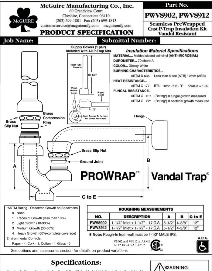
Seamless PreWrapped Adjustable Cast Brass P-Trap Kit furnished with McGuire's Vandal Trap@,Vandal Resistant P-Trap with cleanout, seamless supply riser tube covers, supply angle stop covers, angle stop wheel handle covers and deep box flange.
