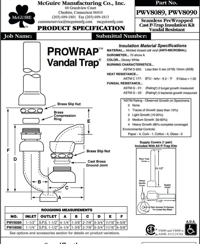
Seamless PreWrapped All Cast Brass Ground Joint Swivel P-Trap Kit furnished with McGuire's Vandal Trap @, Vandal Resistant P-Trap with cleanout and cast brass ground joint elbow. Includes seamless supply riser tube covers, supply angle stop covers and angle stop wheel handle covers.
