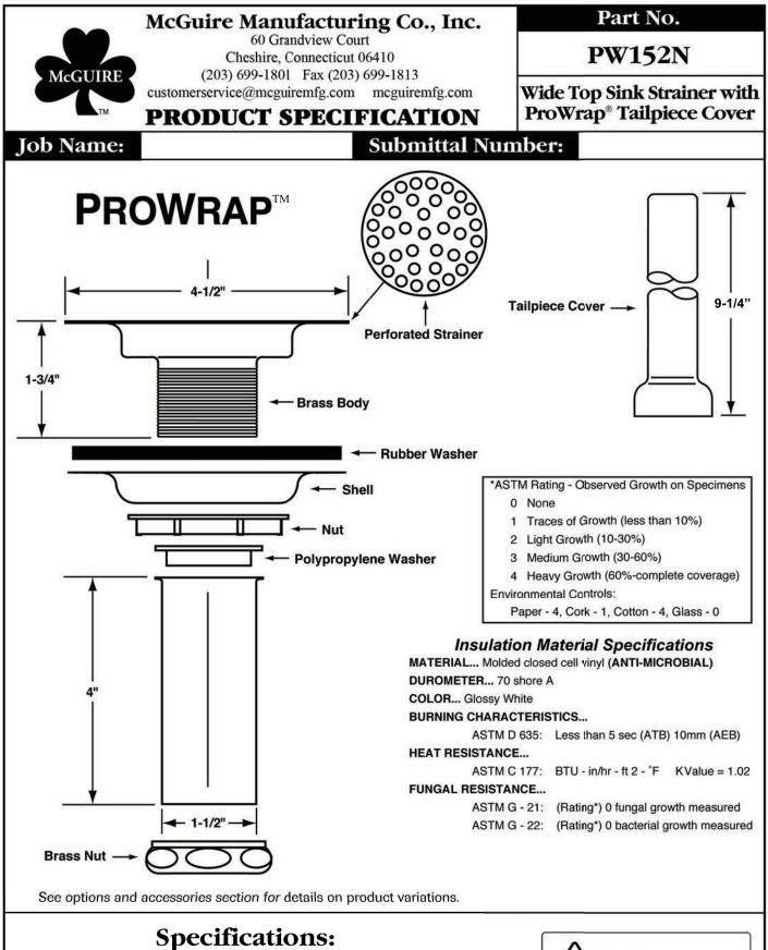
Wrought Brass Chrome Plated Wide Top Sink Strainer with 1-1/2 inch x 4 inch seamless brass tailpiece. Fits sink thickness up to 3/4 inch. Includes seamless ProWrap@ tailpiece cover.
