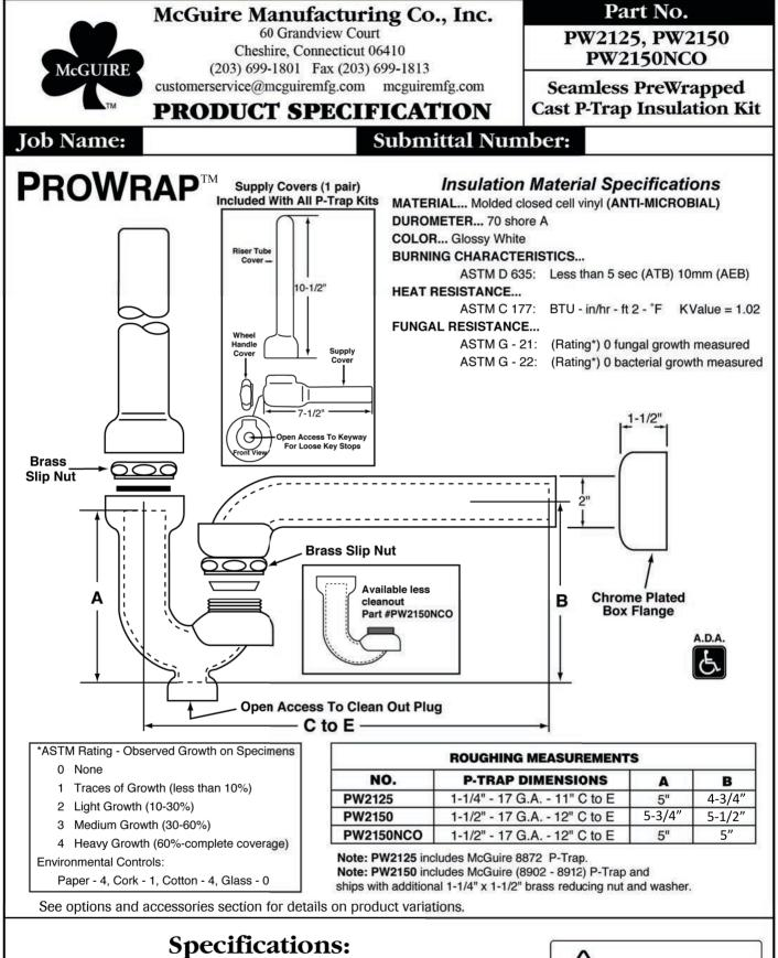
Seamless PreWrapped Adjustable Cast Brass P-Trap Kit furnished with McGuire cast brass adjustable P-Trap with or without cleanout, seamless supply riser tube covers, supply angle stop covers, seamless drain tailpiece cover and angle stop wheel handle covers, and chrome plated box flange.
