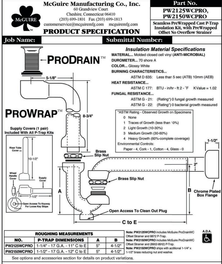
Seamless PreWrapped Adjustable Cast Brass P-Trap Kit with PreWrapped ProDrain@ offset grid drain. Furnished with McGuire cast brass adjustable P-Trap with cleanout, ProDrain@ offset grid drain assembly, seamless riser tube covers, supply angle stop covers, angle stop wheel handle covers, and chrome lated box flange.
