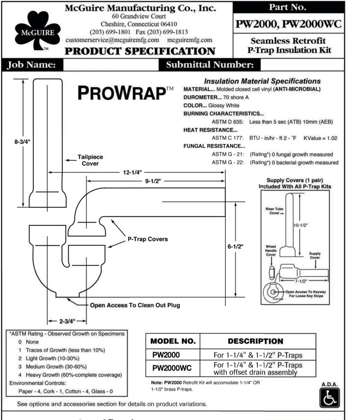
Seamless Retrofit P-Trap Insulation Kit furnished with seamless riser tube covers, supply angle stop covers, seamless drain tailpiece cover and angle stop wheel handle covers.
