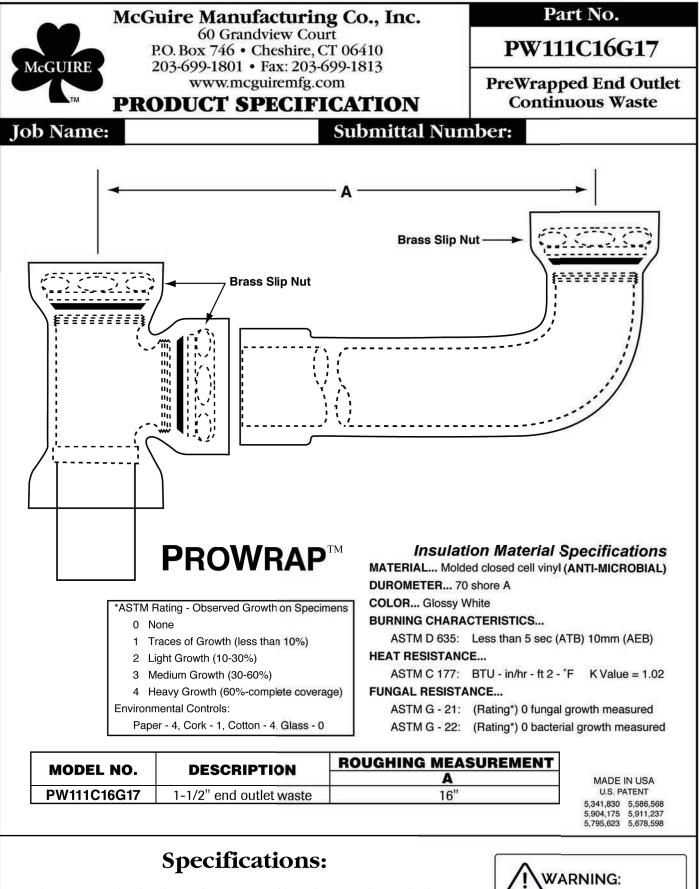
Seamless PreWrapped End Outlet Continuous Waste with cast brass tee, chrome plated 17 gauge seamless brass waste arm, brass tailpiece and brass nuts.
