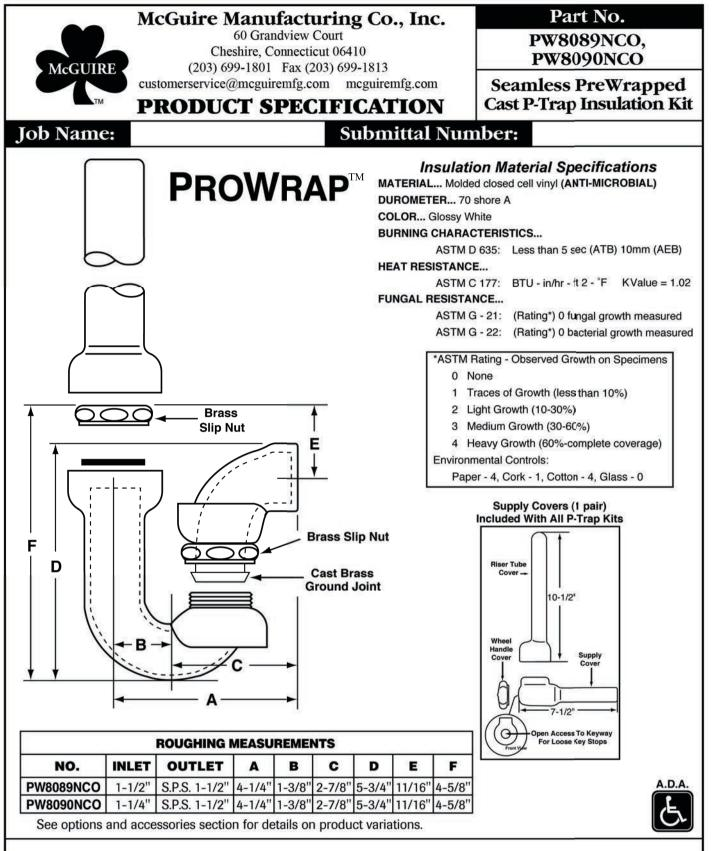
Seamless PreWrappedAll Cast Brass Ground Joint Swivel P-Trap Kit furnished with McGuire cast brass ground joint swivel P-Trap less cleanout, seamless supply riser tube covers, supply angle stop covers and angle stop wheel handle covers.
